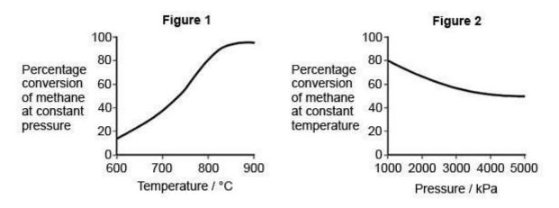
Deduce the optimum conditions for the industrial conversion of methane and steam into the gaseous products.
